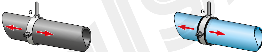
Figure 7.14 Guide point brackets (G).
