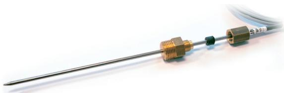
TMW-300 is a water sensor with an adjustable immersion depth. The stainless (rst) Ø 4 mm immersion pipe is 300 mm long. The sensor is used, e.g., as an anticipation sensor in domestic hot water control.
