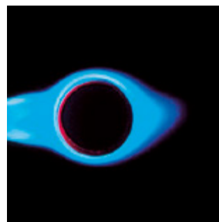
High flame temperature based on cyclone swirl
