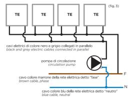
Connection of thermoelectric heads with limit switch contact and circulation pump for heating systems.
