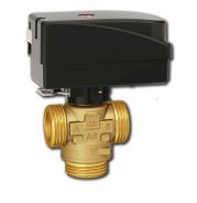
LK 525 MultiZone is a motorized 3-way zone valve for On/Off control. The zone valve is designed with a turning slide which allows it to withstand a larger pressure difference and reduces the risk of it stalling after a long intermission. This makes it especially suited for heat pump applications where there can be long intermissions between the changes to the direction of the flow during the warm season. On the upper surface of the actuator is an indicator that shows which port is open.
