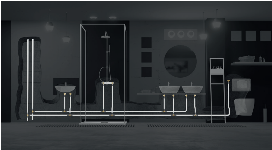
Fig. 42: Single Tee installation.
