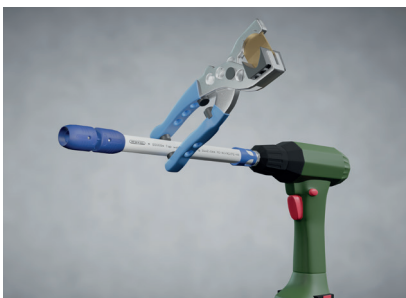
Fig. 23: Calibrating the pipe.
