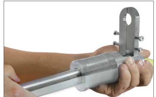
4. Insert the apparatus in the crushing piston and operate a few times on the piston, sliding it out and pressing it in to achieve a sealing surface (flange).
